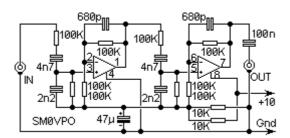
This is a simple filter that restricts the LF response a little as well providing quite a heavy HF roll-off. The prototype has enhanced a Yaesu FT101B that was only fitted with an AM IF filter. The IC is an LM358. Construction needs no detailed description. Layout is not critical.
